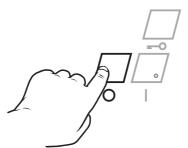
All the cooking zones can be switched off quickly with the OFF-sensor.
